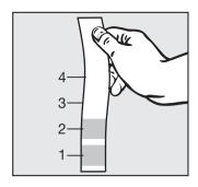
■ Dip the strip in your drinking water for approximately a second, then shake off any excess water. The result will be evident after about a minute.
